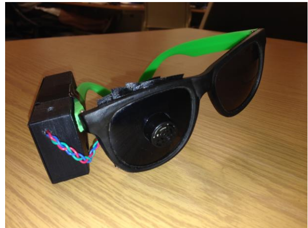
Fig. 2. Finished headset with mounted ultrasonic sensor.
