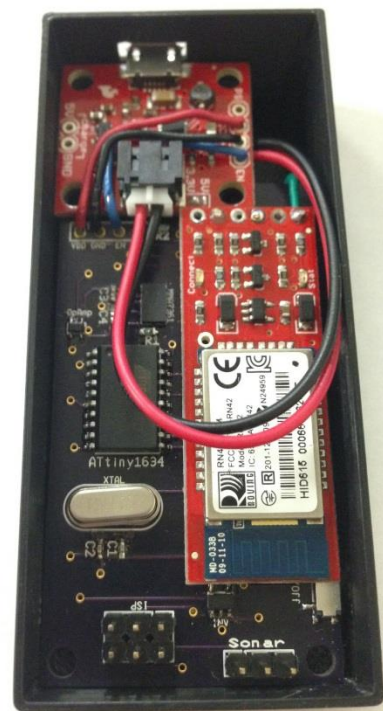
Figure 15.33: Circuit fitted into headset housing.
