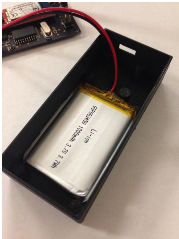
Figure 15.32: Battery fitted into headset housing.
