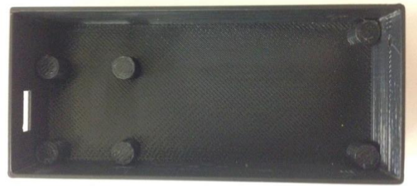
Figure 15.31: 3D-printed headset housing interior.
