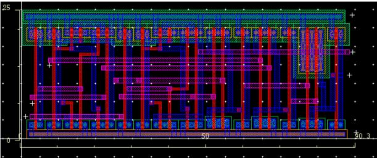
Full Adder Layout (Area \approx 25 \times 90 \mu\text{m} )
